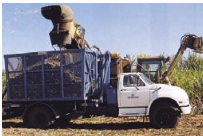
Weighing a mechanically harvested field experiment with a load cell equipped truck.
