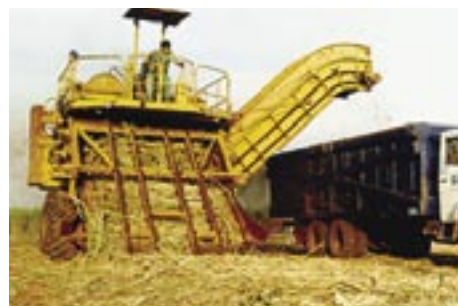
Continuous Loader processing cane and transferring it to the truck.
