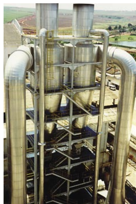
Usina São Martinho, Bagasse dryer and cyclone.
