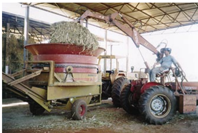
Haybuster machine being fed with trash bales.
