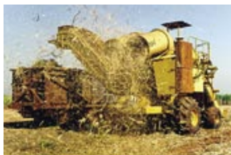
Continuous Loader removing trash and mineral impurities from cane billets.
