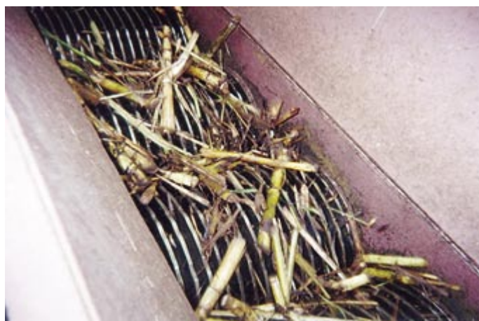
Rotary discs impurities separator.
