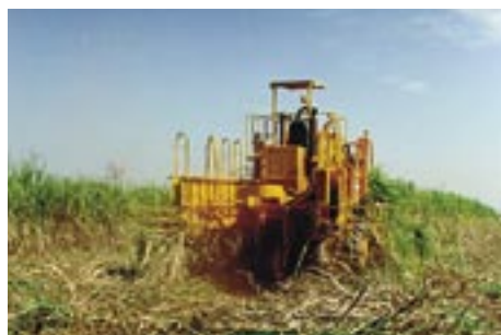
Two-Row Whole Stalk Copersucar Harvester cutting cane.
