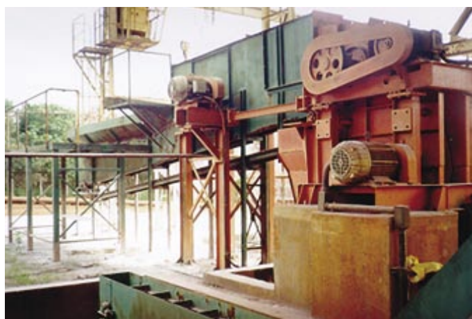
Knife and shredder system at Usina São Luiz AA.
